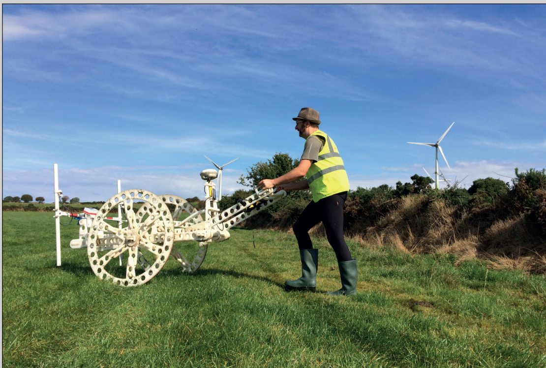
Jonathan undertaking a geophysical survey using dual array fluxgate magnetometer probes on a GPS survey configured cart at Carragraigue, 20ha proposed Solar Farm, near Millstreet, Cork
